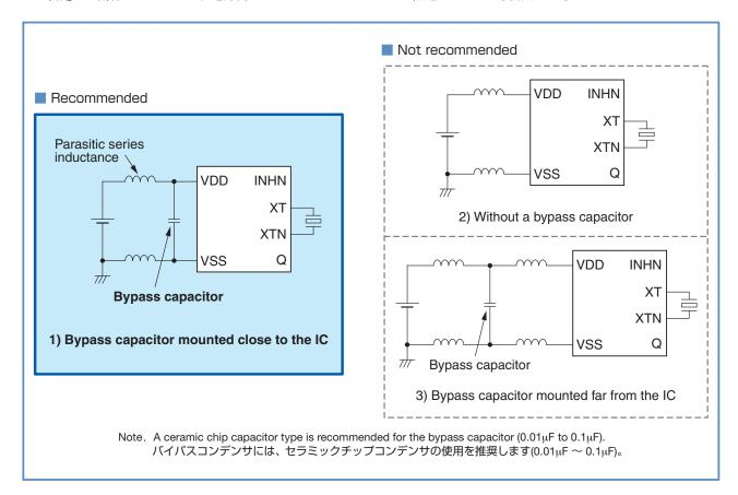
The effectiveness of the bypass capacitor drops as the distance between the IC supply pads and the bypass capacitor increases. This is because, even though noise is reduced by the bypass capacitor, noise can also occur again due to the wiring inductance components. Furthermore, as the oscillation frequency increases, the noise due to inductance components also increases, making the placement of the bypass capacitor very important in high-frequency oscillators.
